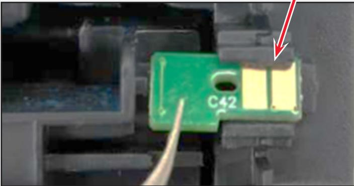
Use tweezers to insert the replacement chip into the slot.
