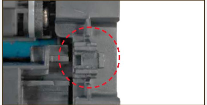
Locate the chip housing area on the cartridge.
