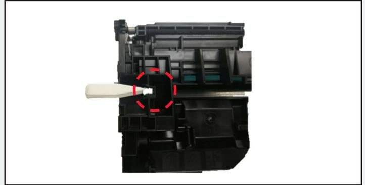
Remove the OEM chip with tweezers.
