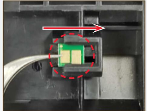
Use the tweezers to insert the replacement chip into the slot as shown by the arrow. Be sure not to install the chip backwards.
