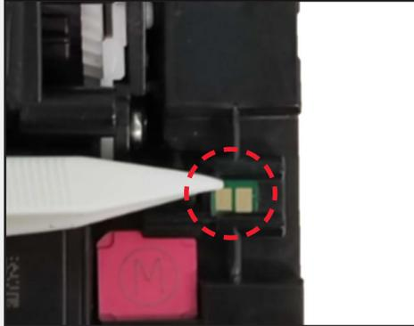
Remove the OEM chip with tweezers.
