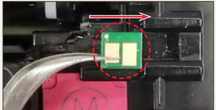
Use the tweezers to insert the replacement chip into the slot as shown by the arrow. Please do not install backwards. If the chip is loosely installed, it will need to be fixed with glue.
