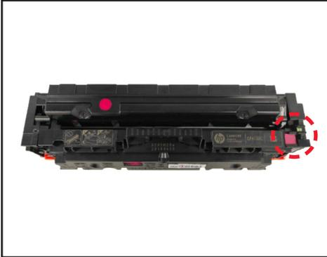
Locate the used chip on the cartridge.
