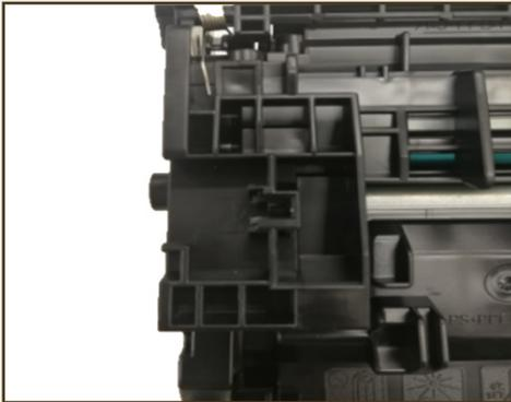
Here is the cartridge after removing the OEM chip.
