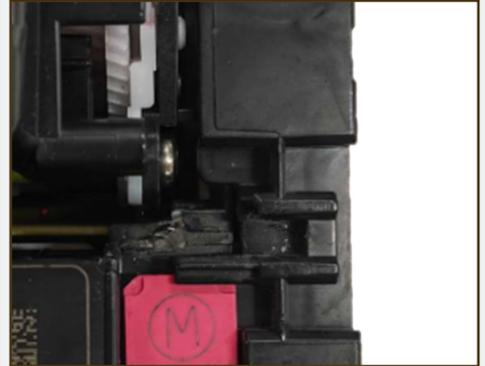
Here is the cartridge with no chip installed.
