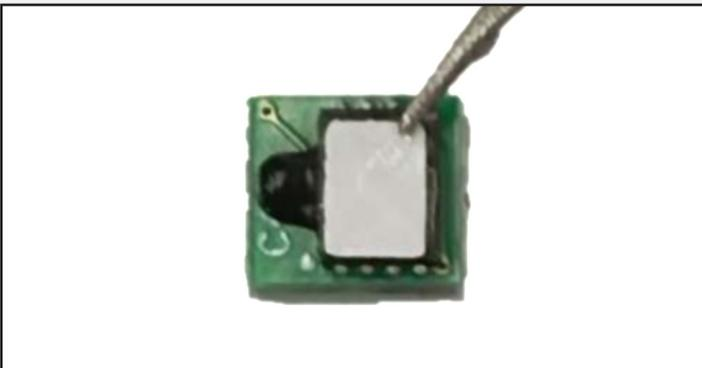
Use insulated tools to peel the adhesive off the replacement chip.
