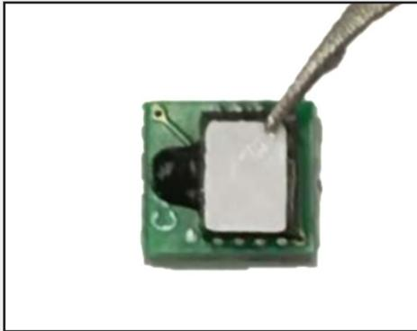
Carefully peel the adhesive off the replacement chip.
